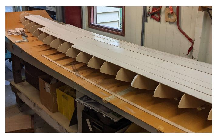
Figure 3.7: Attaching the deck skin to the mould frame.
