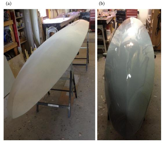
Figure 4.52: (a) After primer coats and (b) after final overcoat.
