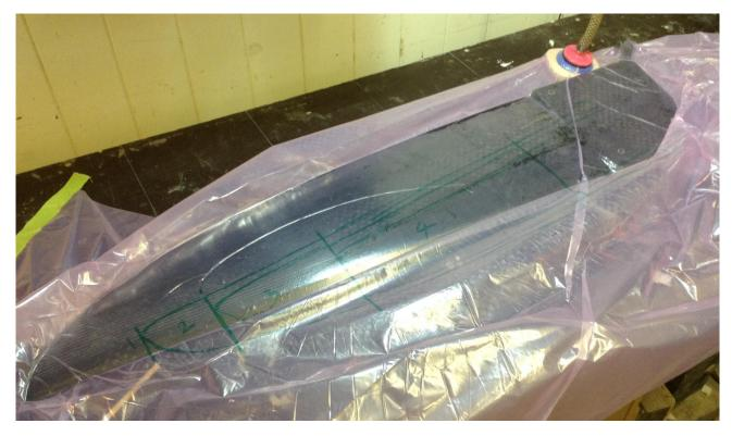
Figure 5.16: Gluing the two halves together under vacuum.
