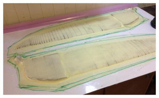
Figure 5.9: Thickened epoxy and layers of fibreglass applied over the positive half moulds. The fibreglass extends beyond the moulds to form a flange.
