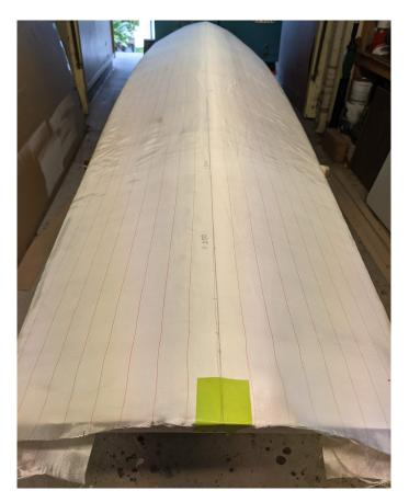
Figure 4.3: Peel ply against the mould.
