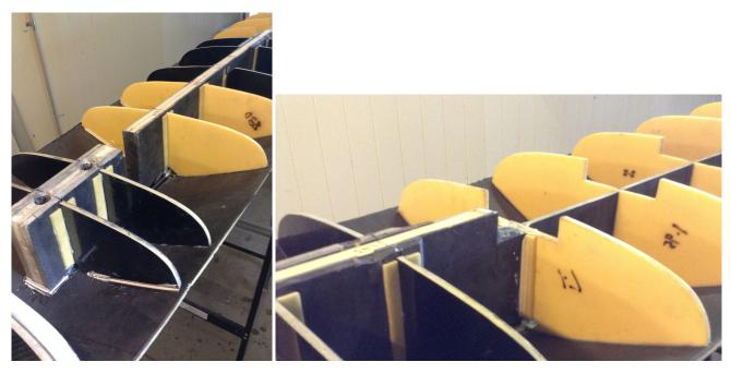
Figure 4.27: Centre-board box and fin box glued into hull.
