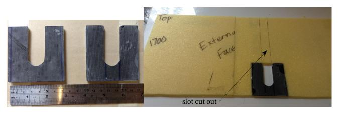
Figure 4.13: Slots for centre-board pivot point, where the slot in the HDF has not yet been cut out.
