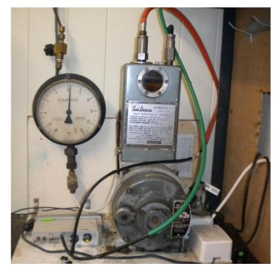
Figure A.1: Vacuum system showing the pressure gauge and electronic vacuum regulator.
