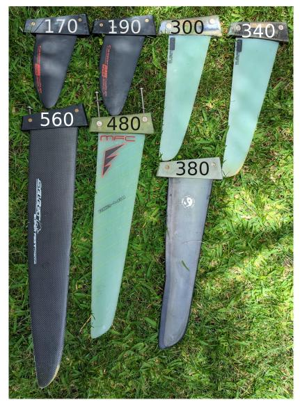
Figure 6.7: Range of different fins, the 300 mm fin seems about right.
