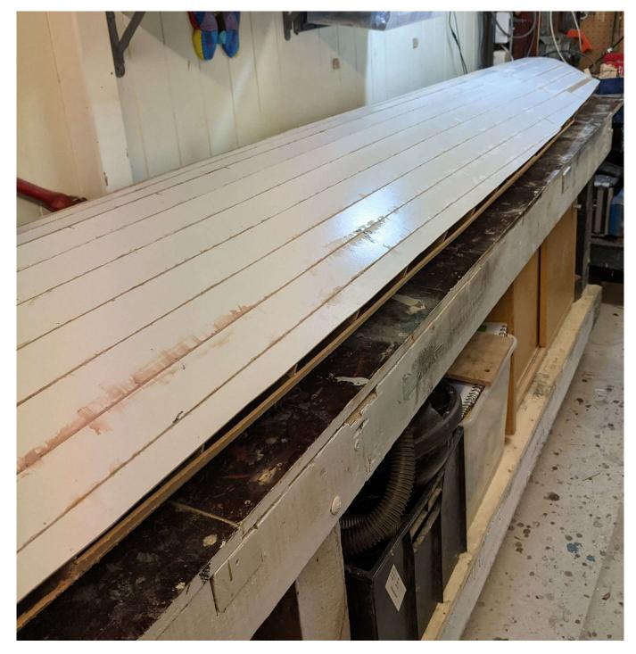
Figure 3.11: Almost finished attaching hull skin to the mould frame.
