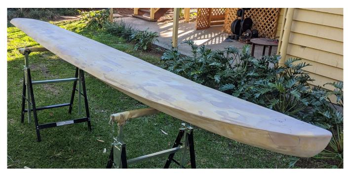
Figure 3.17: Plaster covered mould with bow piece faired in.
