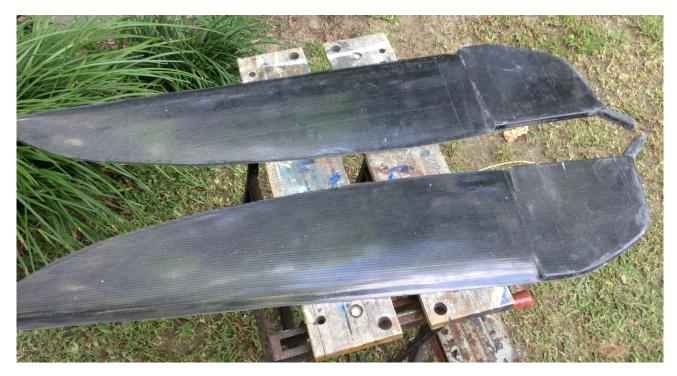
Figure 5.14: Centre-board halves after demoulding.
