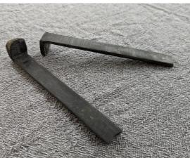
Figure 5.19: Guide strip to restrain centre-board pivot pin.
