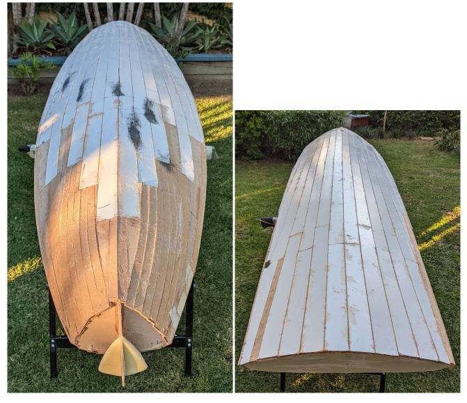
Figure 3.13: Finished attaching MDF skin to mould frame.
