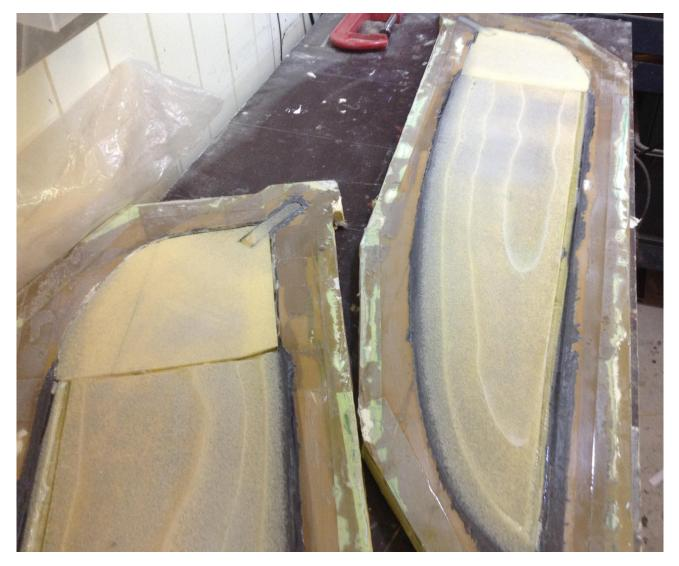
Figure 5.13: Further layers of HDF added to the core and sanded level with mould flange.
