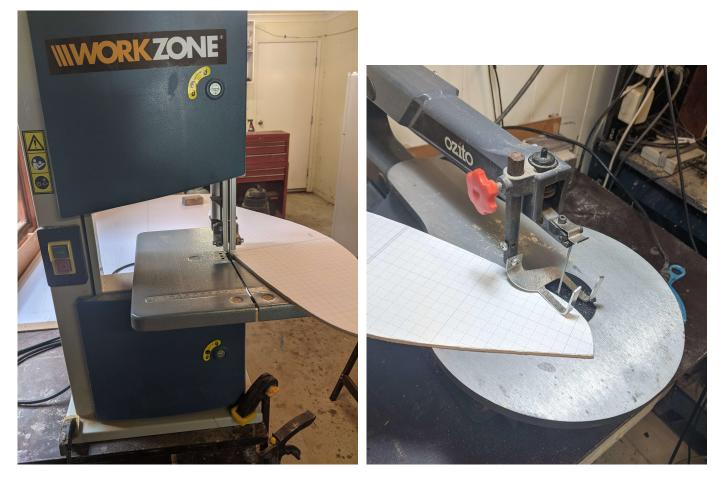
Figure 3.2: Mostly used a bandsaw (a) to cut the profiles. For tighter curves the scrollsaw (b) was useful but not essential.
