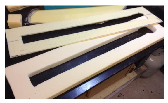
Figure 4.21: Foam pieces used to create a mast track cavity.
