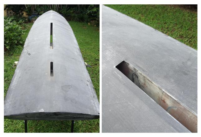
Figure 4.46: Slots for the fin and centre-board cut open (viewed from hull side.
