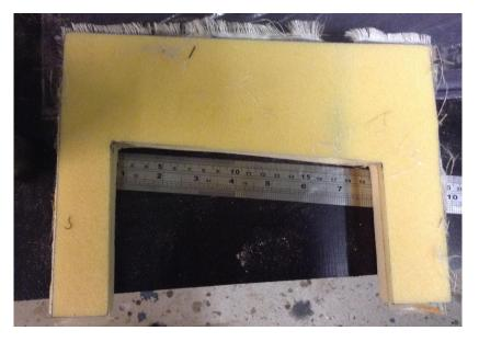
Figure 4.17: Foam shaped to fit around the Tuttle fin-box.
