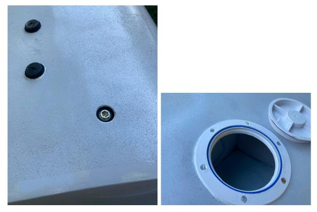
Figure 6.4: Vent plug, fin bolt hole end caps, and inspection hatch.
