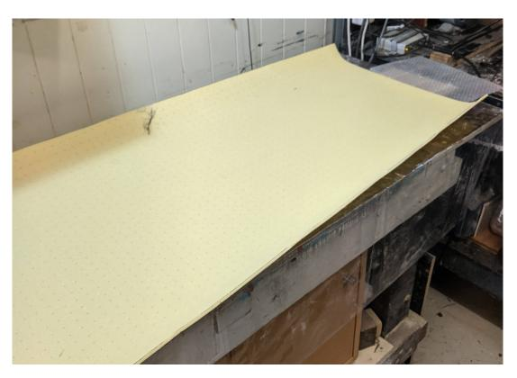
Figure 4.2: Deck foam after pre-bending it.
