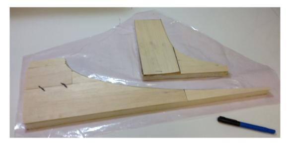
Figure 4.14: PU foam with a balsa shim used to separate the centre-board box panels.
