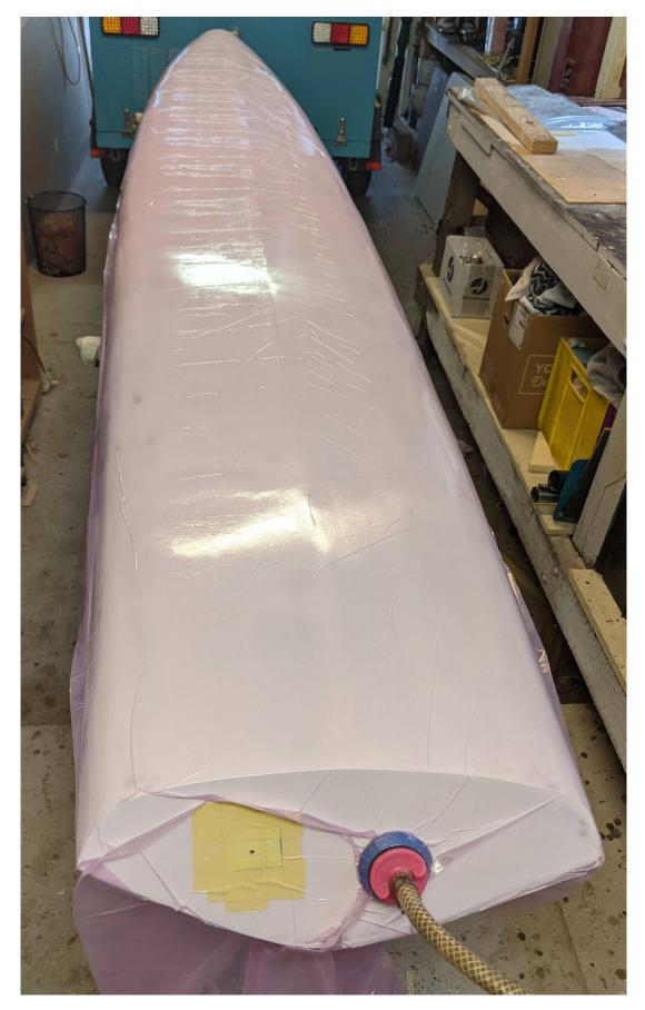
Figure 4.1: Leak check of vacuum bag and mould, showing the vent (left) which ensures the inside of the mould is at atmospheric pressure and the vacuum hose (right).
