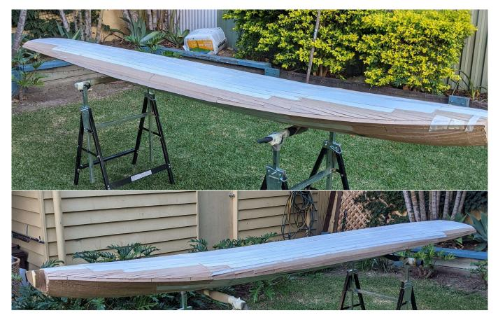
Figure 3.12: Finished attaching MDF skin to mould frame.
