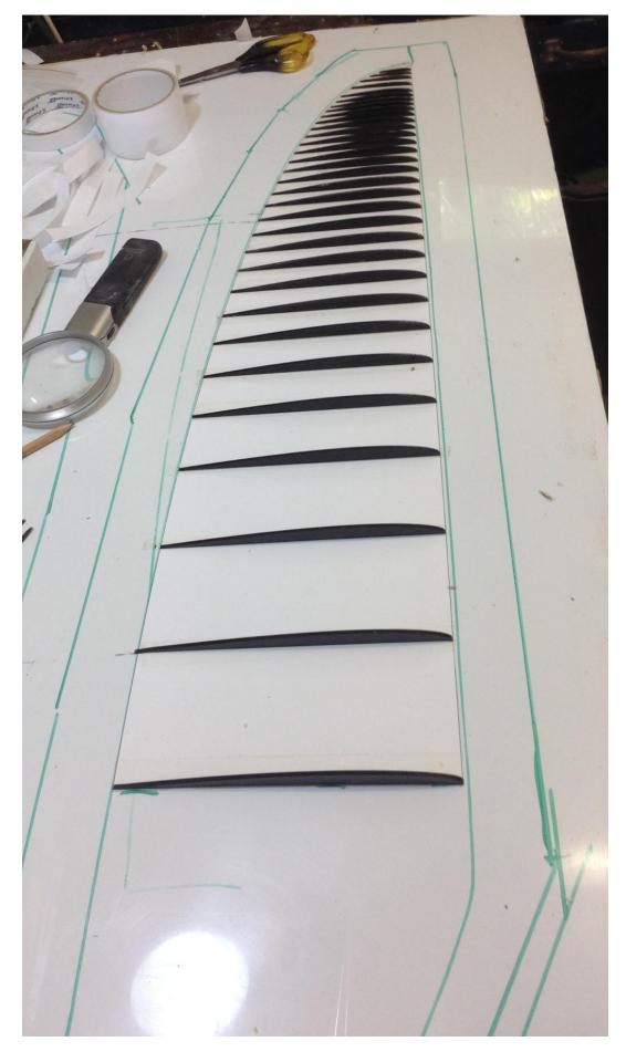
Figure 5.7: Half-sections aligned on the planform template.
