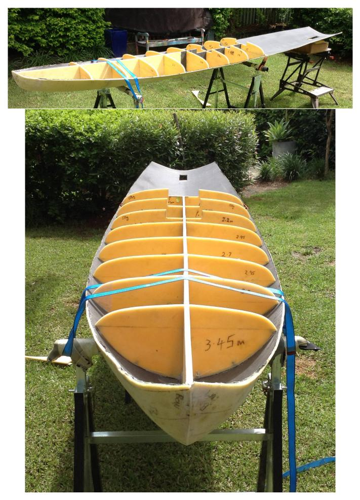
Figure 4.26: Front stringer and bulkheads glued into hull.
