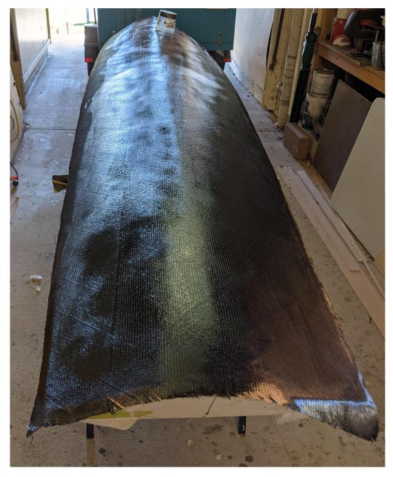
Figure 4.8: Laying up carbon onto the mould.
