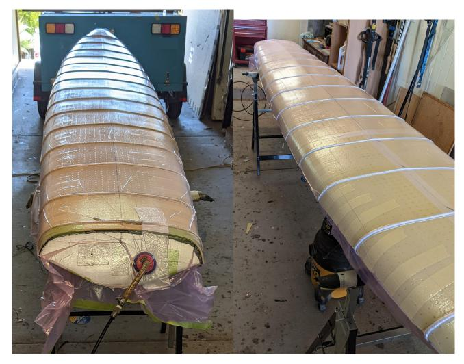
Figure 4.4: Deck inside the vacuum bag.
