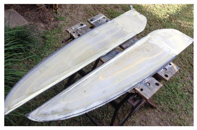
Figure 5.15: Centre-board halves after demoulding.
