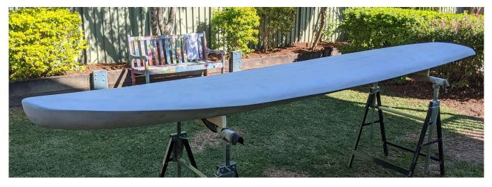
Figure 3.19: Finished mould.
