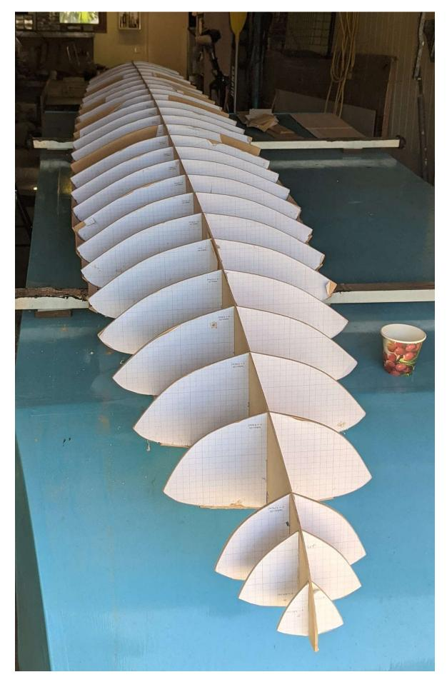
Figure 3.8: View of mould frame after some deck skin has been attached.
