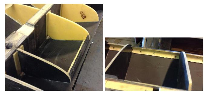
Figure 4.31: Chine bracket inserted between bulkheads, the temporary screws were used to clamp parts while glue dried.
