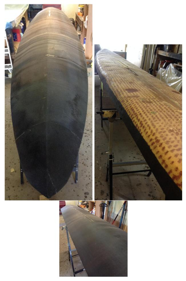
Figure 4.43: Hull outer carbon lamination and showing lamination rapped around onto deck.
