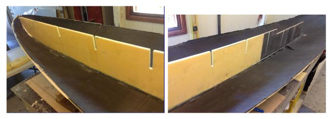
Figure 4.25: Front stringer glued into the hull, note cut-out in carbon section for the mast-track box.
