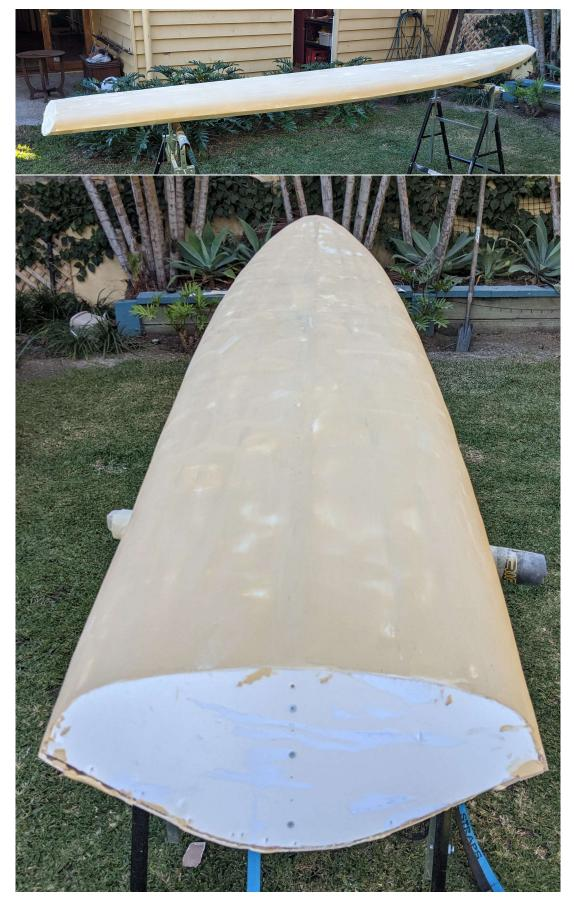
Figure 3.15: Plaster filler added to mould.
