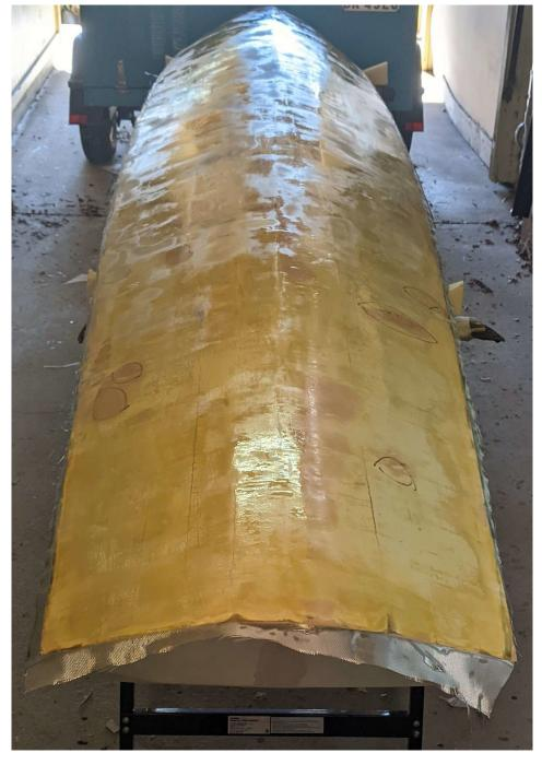
Figure 3.18: Sheathing mould with fibreglass.
