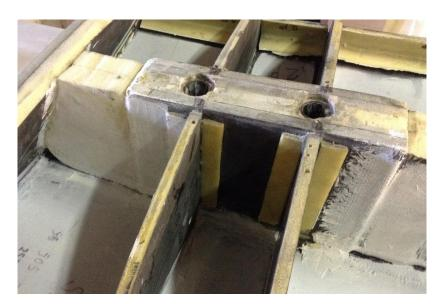
Figure 4.30: PU foam and fibreglass was used to tie the fin-box to the forward and aft structures.
