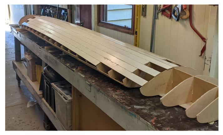
Figure 3.9: Attaching the hull skin to the mould frame.
