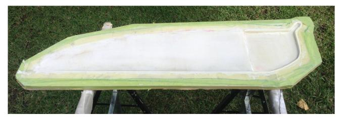
Figure 5.10: Completed port-side negative mould.
