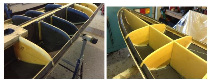
Figure 4.32: Installed chine sections.
