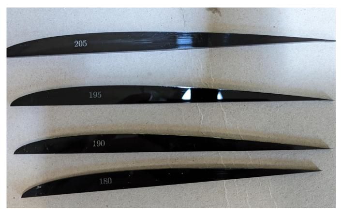
Figure 5.5: Some of the laser cut half-sections used to construct the positive mould. The chord length was engraved on each section when they were laser cut.
