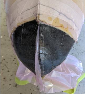
Figure 4.9: Hull inside the vacuum bag.
