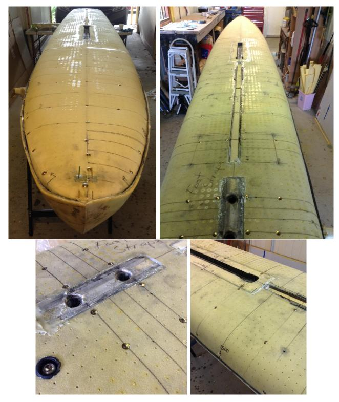
Figure 4.38: Deck glued to frame and hull assembly with temporary screws.
