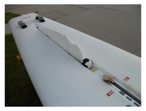
Figure 5.1: Retracted centre-board on an original Lechner.
