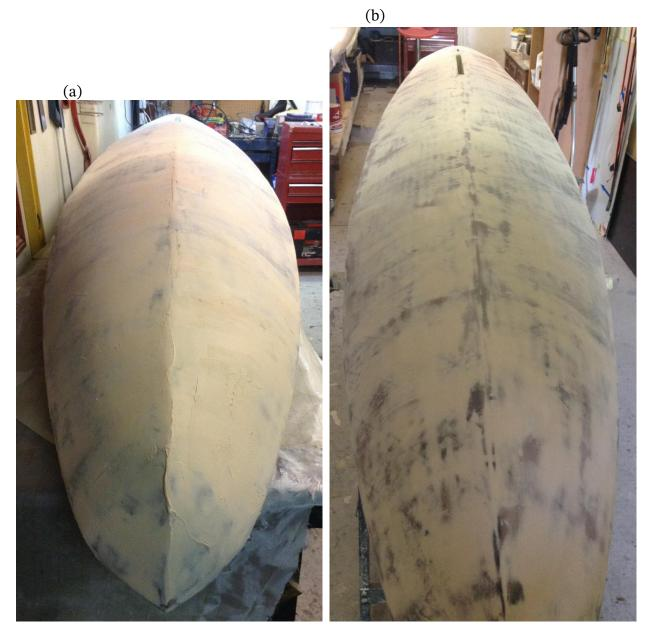
Figure 4.47: (a) High build epoxy surfacer was used to fill the weave. (b) After sanding
