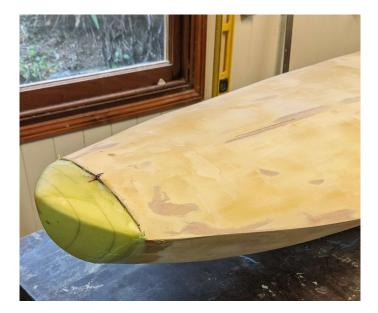
Figure 3.16: Bow shaped using polyurethane (PU) foam.
