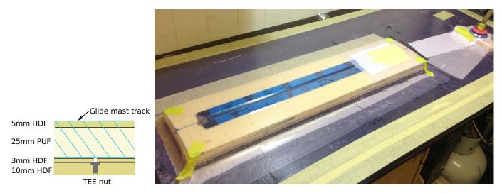
Figure 4.22: Layup of mast track box and mast track box under vacuum.
