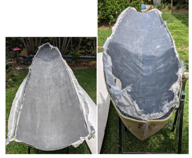
Figure 4.10: Demoulded hull but with peel ply still attached.
