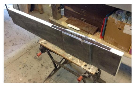
Figure 4.15: Completed centre-board box view from top starboard.
