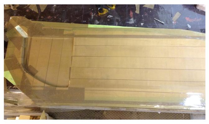
Figure 5.11: Negative mould surface prepared
