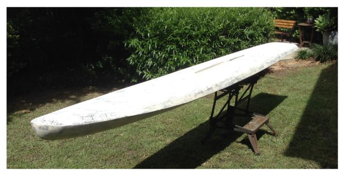
Figure 4.48: The weave has been filled and imperfections filled and faired.
