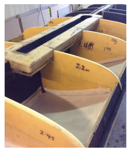
Figure 4.33: Mast-track box installed.
