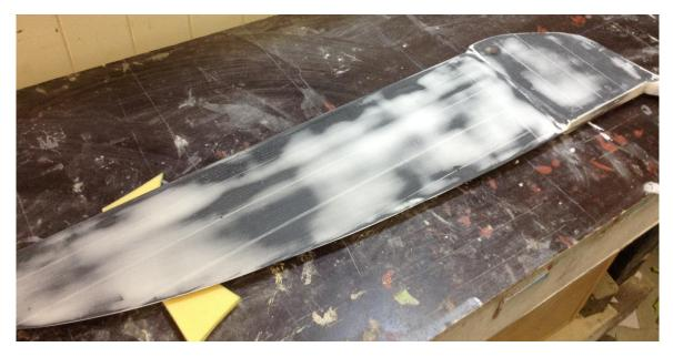
Figure 5.17: Centre-board after some filling and sanding.
