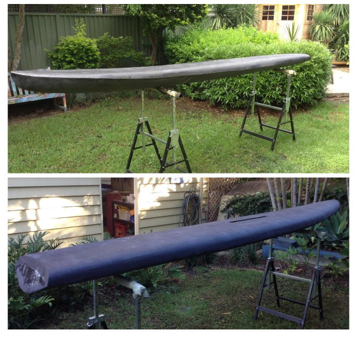
Figure 4.45: Deck outer carbon lamination and showing lamination rapped around onto stern.
