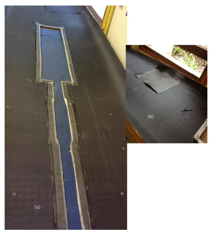
Figure 4.35: (a) Deck cut-out for mast-track and centre-box, showing fibre-glass "skirt". (b) Extra layer of carbon fibre at location of deck hatch.
