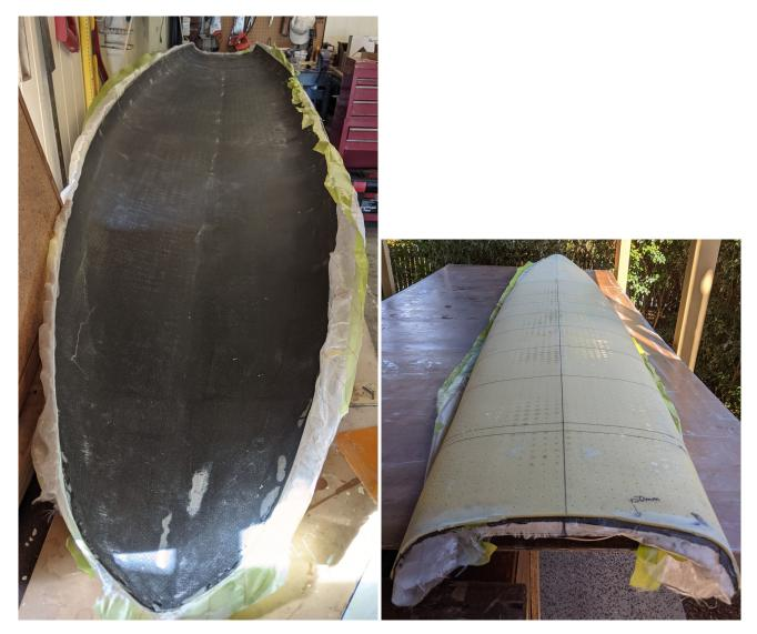
Figure 4.5: Deck demoulded, with peel ply still attached.
